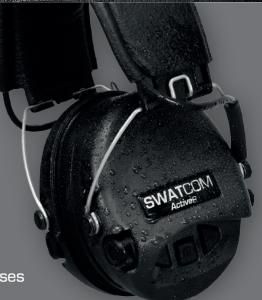
The electronic design utilises the ASIC (Application Specific Integrated Circuit) circuit and is controlled by a microprocessor. This makes it possible to combine very low current consumption with high performance and instead of cutting off peak sounds it compresses them down to a safe level of 82 dB(A).
