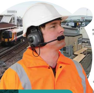
Whether you choose our comfortable over-the-head or convenient hard hat compatible styles, Apex headsets allow hands-free, full-duplex communication and are fully programmable with your choice of a three-way toggle switch or push-to-talk button. A noise-cancelling electret microphone comes mounted on a flex-style boom for left or right dress, and transmits up to 600 metres with unparalleled clarity, even in extremely noisy environments.
